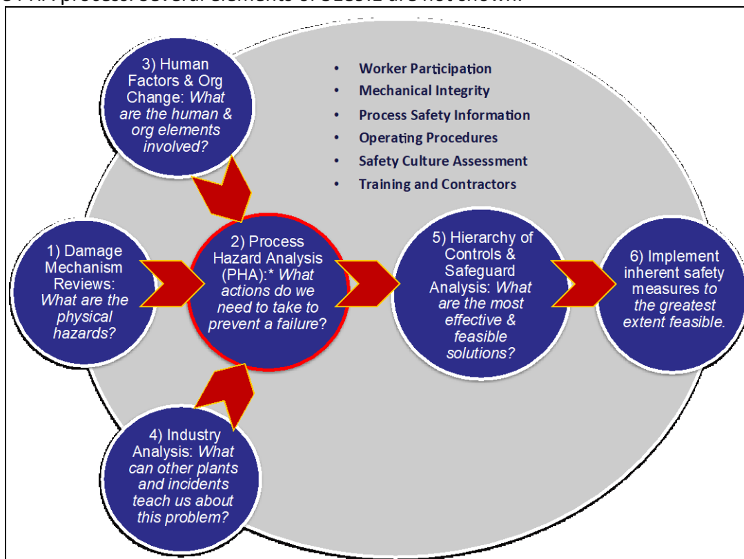
Figure 1. Graphic illustration of section 5189.1. Section 5189 requires the PHA but does not require the preliminary and subsequent elements shown. Each of the bulleted elements is integrated into each step of the PHA process. Several elements of 5189.1 are not shown.
