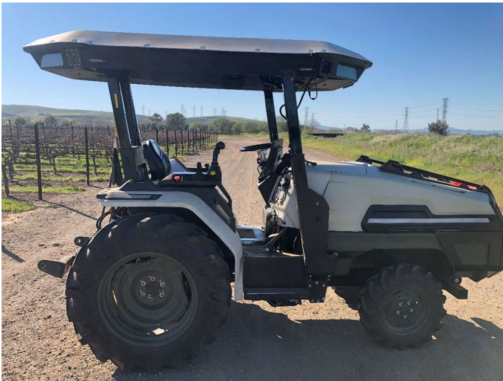
Figure 1. Monarch Tractor, with cameras mounted on the roll-over protection roof.
