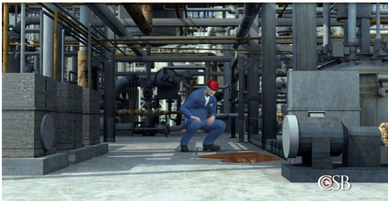
Figure 6. CSB animation depicting operator identifying the leaking 4-sidecut pipe.
