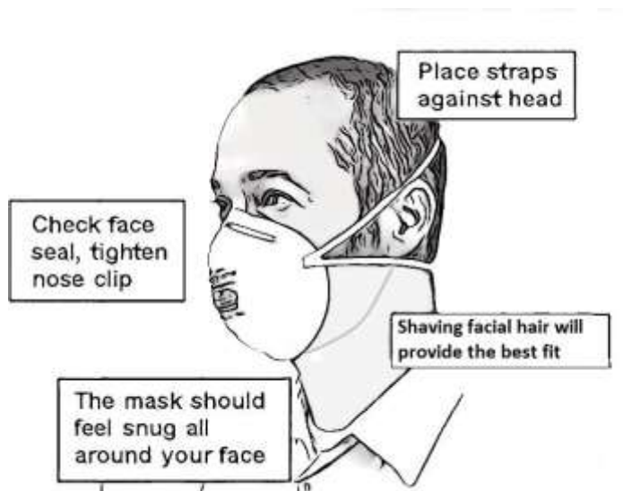
Drawing Showing Proper Fitting of a Filtering Facepiece Respirator (shaving is not required for voluntary respirator use)
