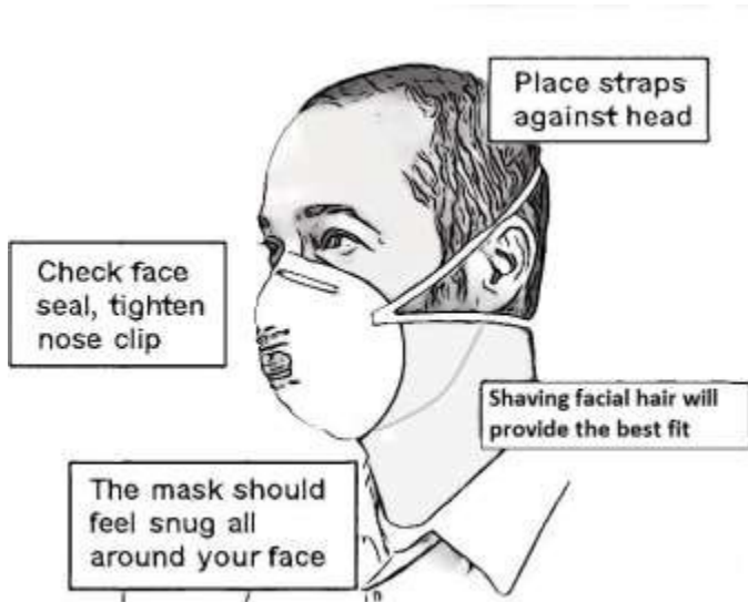
Drawing Showing Proper Fitting of a Filtering Facepiece Respirator (shaving is recommended but not required for voluntary respirator use)
