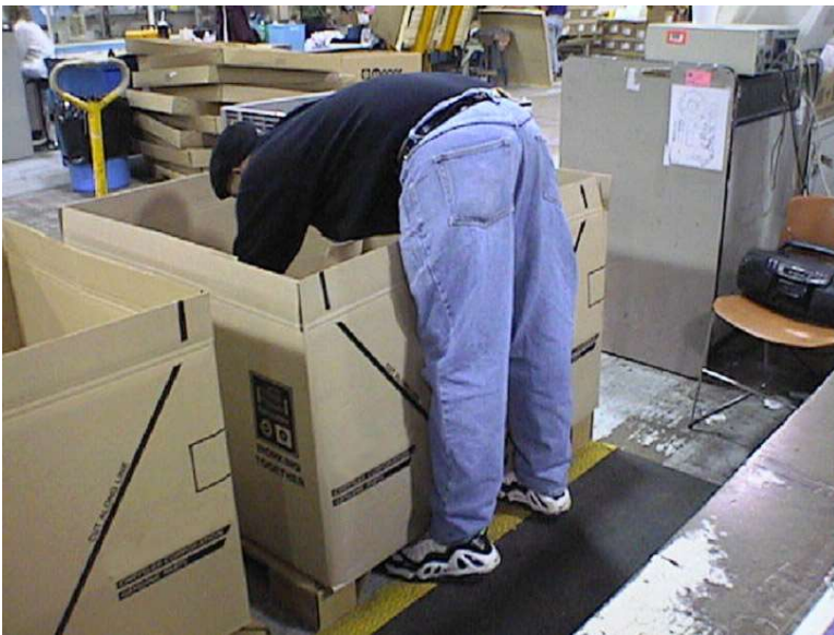
Figure 5: As is readily apparent, this is a highly awkward lifting task. Moreover, cardboard tri-wall containers add to back stress because they do not allow workers to brace against the wall of the container when lifting 4 .
