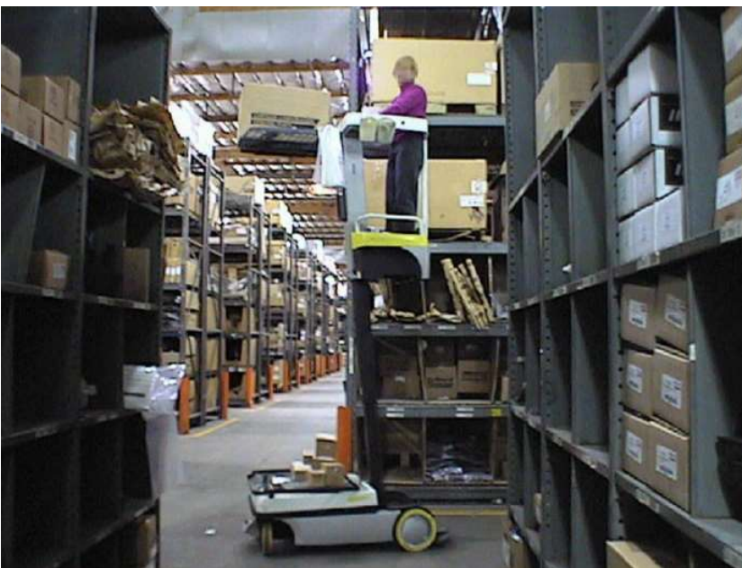
Figure 6b: Picture shows the same job depicted in 6a after new equipment was used to raise workers to the proper height to retrieve small boxed parts.
