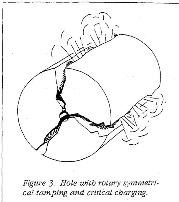
Figure 3. Hole with rotary symmetrical tamping and critical charging.
