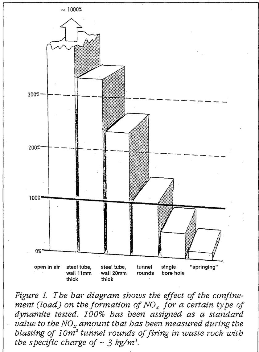
Figure 1. The bar diagram shows the effect of the confinement (load) on the formation of  $\text{NO}_x$  for a certain type of dynamite tested. 100% has been assigned as a standard value to the  $\text{NO}_x$  amount that has been measured during the blasting of  $10\text{m}^2$  tunnel rounds of firing in waste rock with the specific charge of  $\sim 3\text{ kg/m}^3$ .
