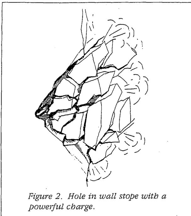
Figure 2. Hole in wall stope with a powerful charge.
