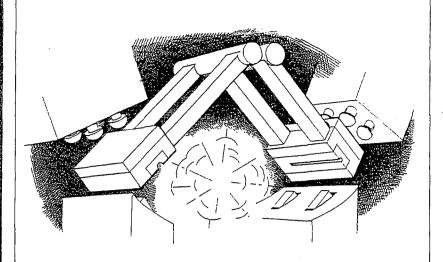
Figure 6. Proposal for a twin pendulum for charge energies up to 10 MJ. Note the hydraulic shock absorbers, the hooking-up device, the replaceable loads and steel linings. The sketch is schematic. The contact surfaces (operating surfaces) are provided with labyrinth tracks (grooves) in order to reduce the gas loss between the surfaces during the initial phase.
