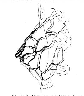
Figure 2. Hole in wall stope with a powerful charge.
