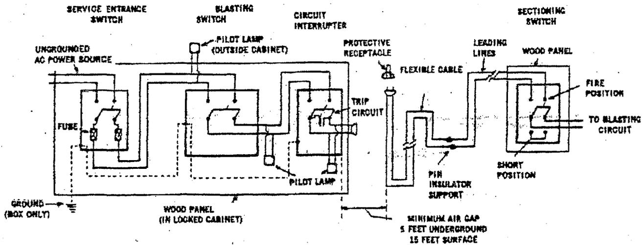
Recommended power firing systems for series and parallel series firing using a circuit interrupter.
