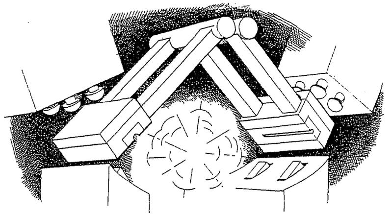
*Figure 6. Proposal for a twin pendulum for charge energies up to 10 MJ. Note the hydraulic shock absorbers, the hooking-up device, the replaceable loads and steel linings. The sketch is schematic. The contact surfaces (operating surfaces) are provided with labyrinth tracks (grooves) in order to reduce the gas loss between the surfaces during the initial phase.*
