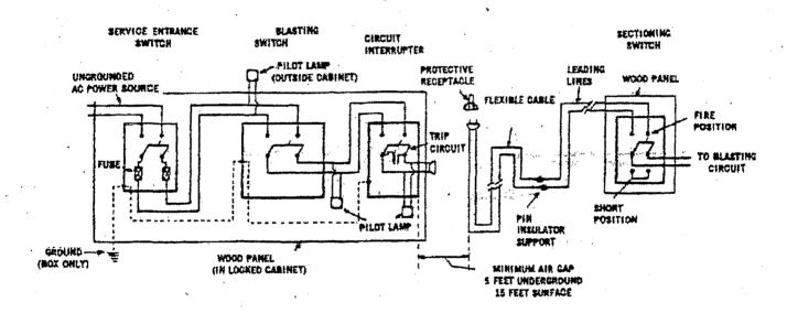
Recommended power firing systems for series and parallel series firing using a circuit interrupter.
