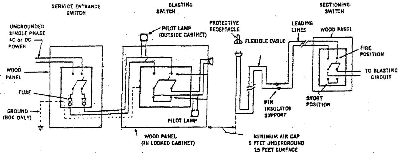
Recommended power firing systems for series and parallel series firing with no circuit interrupter.
