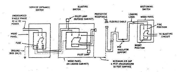
Recommended power firing systems for series and parallel series firing with no circuit interrupter.
