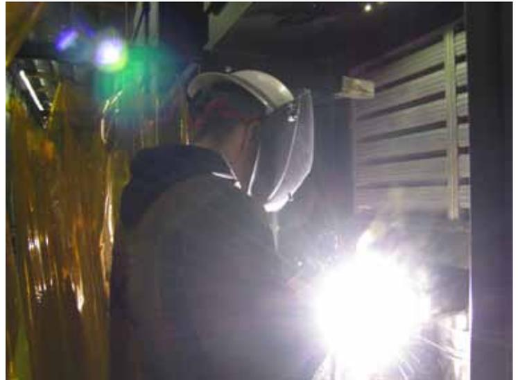
Each weld station accommodates an individual welder and includes a roomy, well lighted work station, articulating fixtures, and a multi-process welding machine.
