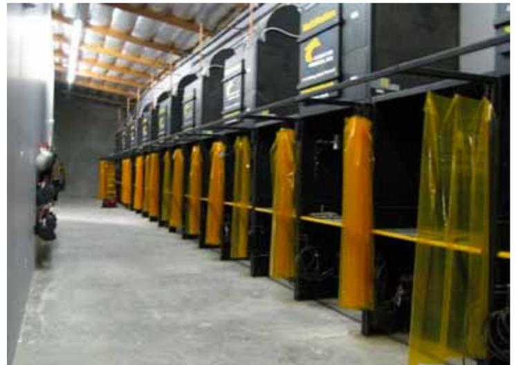
The new Hayward weld booths have individual on-board HEPA air filtration systems which back-draw and process the weld fumes and return the clean air back into the room.
