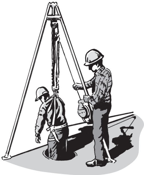
Illustration 3 | Retrieval Equipment in Use
