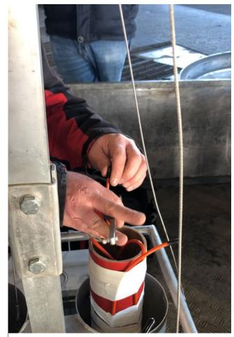
2 minutes to attach four igniters to fuses.
