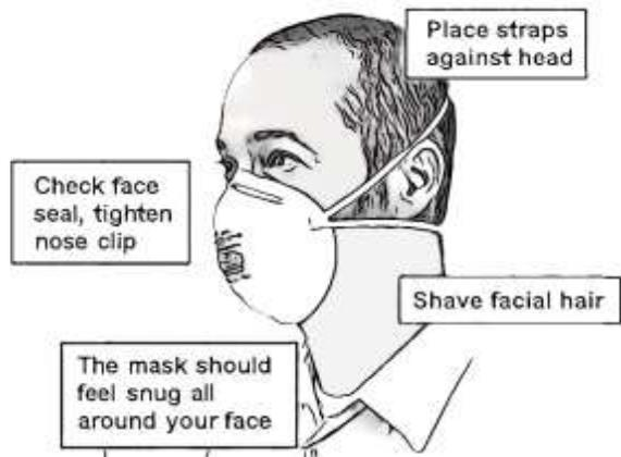
Regardless of the type of respirator, check how well it seals to the face by following the manufacturer's instructions for user seal checks. Adjust the respirator if air leaks between the seal and the face. The more air leaks under the seal, the less protection the user receives.
