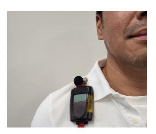
Dosimeters measure and average the noise levels that exceed specified threshold levels. A threshold level is the sound pressure level above which a noise dosimeter begins measuring. The threshold level is set at:
