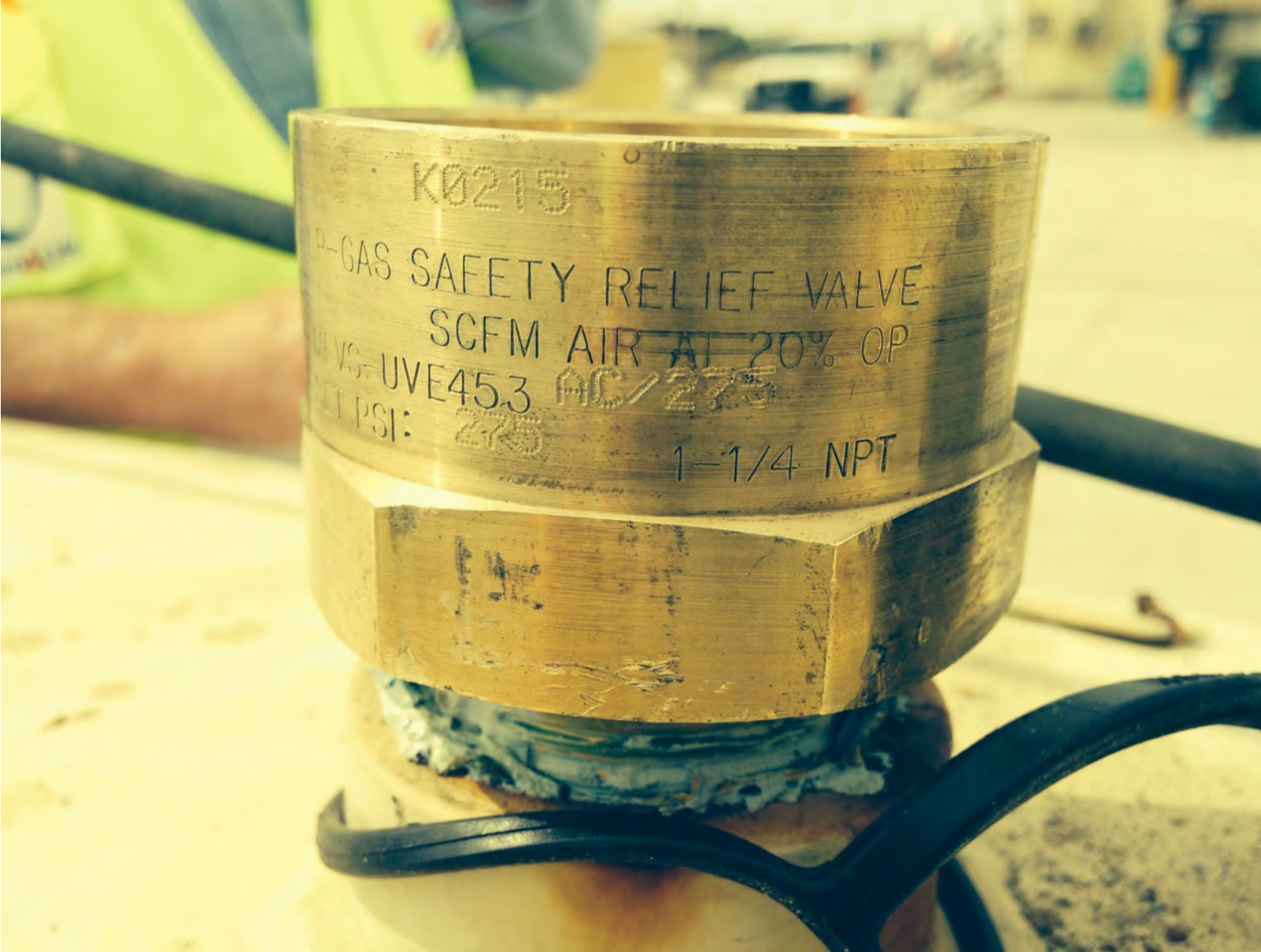
Marshall Excelsior Company – SCFM valve capacity is missing.
