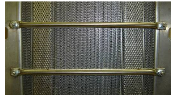
Burner Element – Detail View
