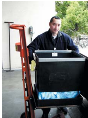
Remove the container from the compacted garbage.
