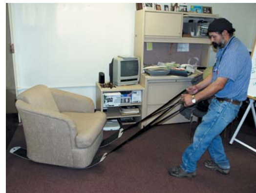
Devices for reducing friction help to easily move heavy furnishings over vinyl, tile, and carpet.
