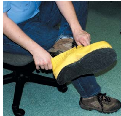
Wear stripping shoes when stripping wax from a floor.
