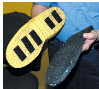
Wear stripping shoes when stripping wax from a floor.
