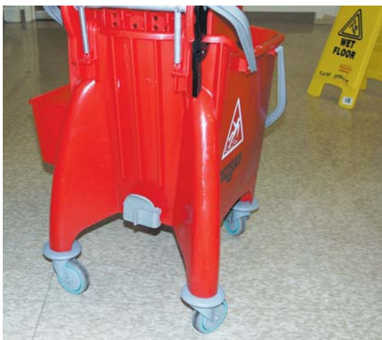
A wide base adds stability to a tall mop bucket.
