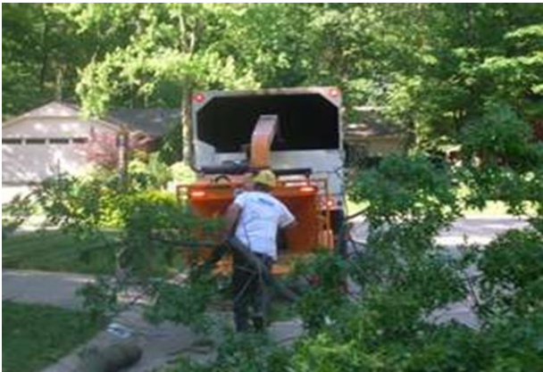
Employee carrying a tree branch for chipping. Load the chipper from the side of the feed, instead of the front.
