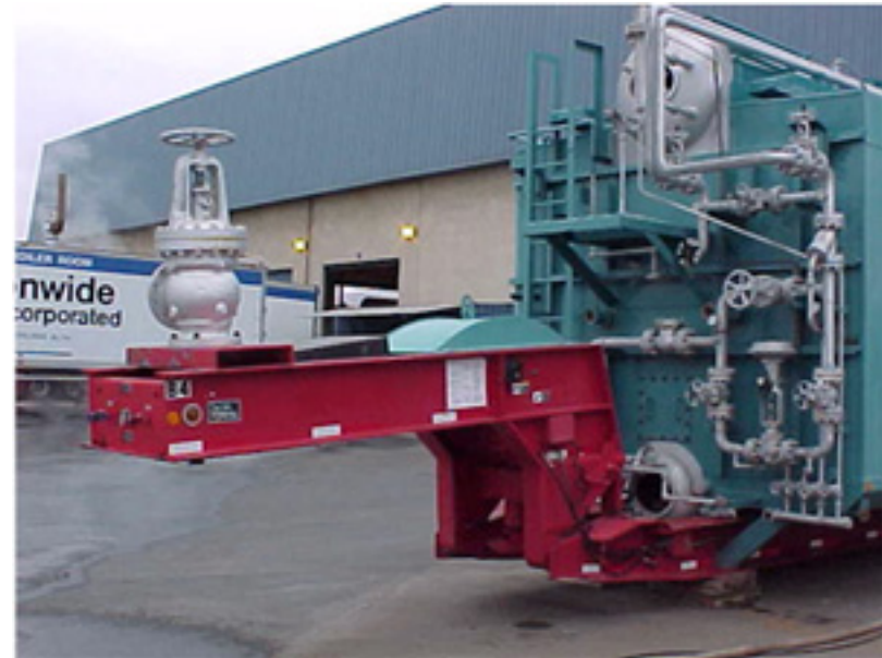
70,000 lb/hr Trailer-Mounted Boiler Front Tow End
