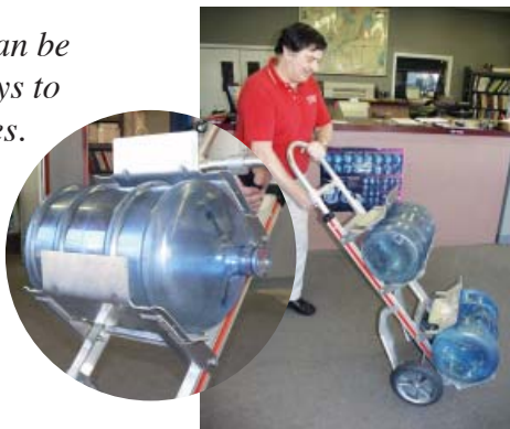
Two-wheel hand trucks work well for transporting bottles or cylinders over short distances.
