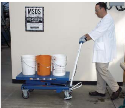
This scissors lift has a foot pump to raise or lower the platform so the containers can be slid on or off.
