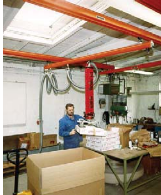
A workstation crane fitted with a balancer and a vacuum lifter for handling large or heavy containers
