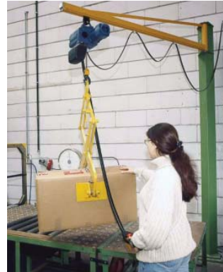
A jib crane fitted with an electric hoist and a lifting tong
